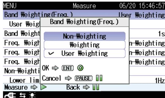
Sets the frequency weighting characteristics for a specific band.
