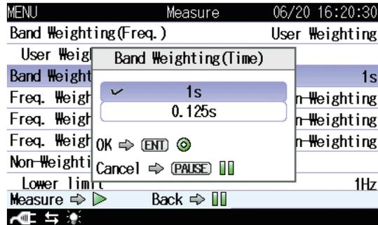
The time weighting setting is reflected in the Inst and Calc Max values, but not in the AP, AP(W), and Calc values.
