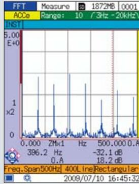
When diagnosing a bearing fault, it is necessary to know the repeat cycle of the impact waveform. This can be achieved by envelope processing, using the principle illustrated below.
