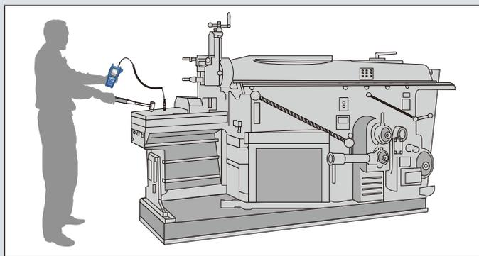
To measure the resonance frequency, the structure is struck with a hammer or similar and the resulting vibrations are subject to frequency analysis.
