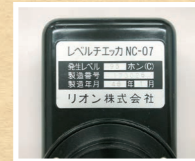
② The name of the product, manufactured in 1973, is the Sound Level Checker. It produces a 95-phon sound—a phon being a unit used for sound levels in those days. Let's take it apart, shall we?
