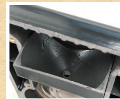
④ Here's the hole through which the sand is to fall. It's indeed shaped like an hourglass. The hole is about 2 mm in diameter.
