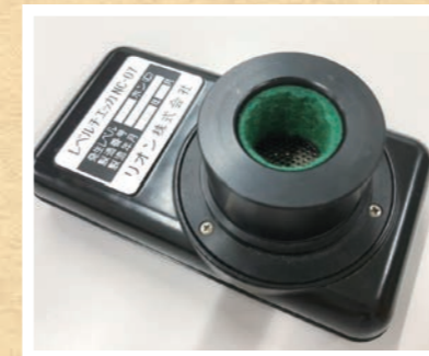
① The early models are now regarded as antiques. This is the NC-07, one of the later models we discovered at the workplace. It has a port for a 1-inch microphone.
