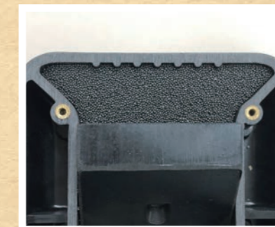
⑤ This is what the instrument looks like when it's filled with sand. Since the cover is removed, we have to be careful to avoid spilling the sand.
