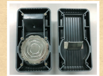
③ Here's a view of the interior. On the left is the front panel; on the right is the back panel. The circular metal plate on the left panel must be the resonator. (The sand has been removed.) As you can see, the design is starkly simple.
