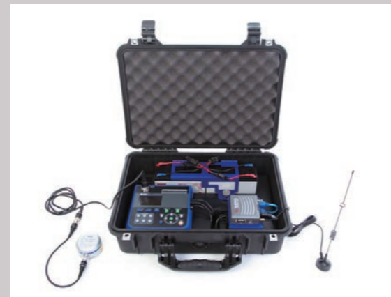
a Live to Web system based upon the Rion XV-2P vibration meter
