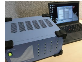
Measuring reverberation time (SA-02M, AS-20PC5)
