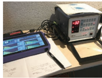
Measuring sound insulation (RIONOTE, SF-06)
