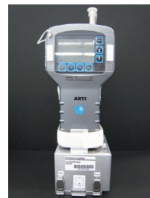
Figure 1 ©JAXA : Modified particle counter. The box at the bottom is a dry cell box attached as a modification.
