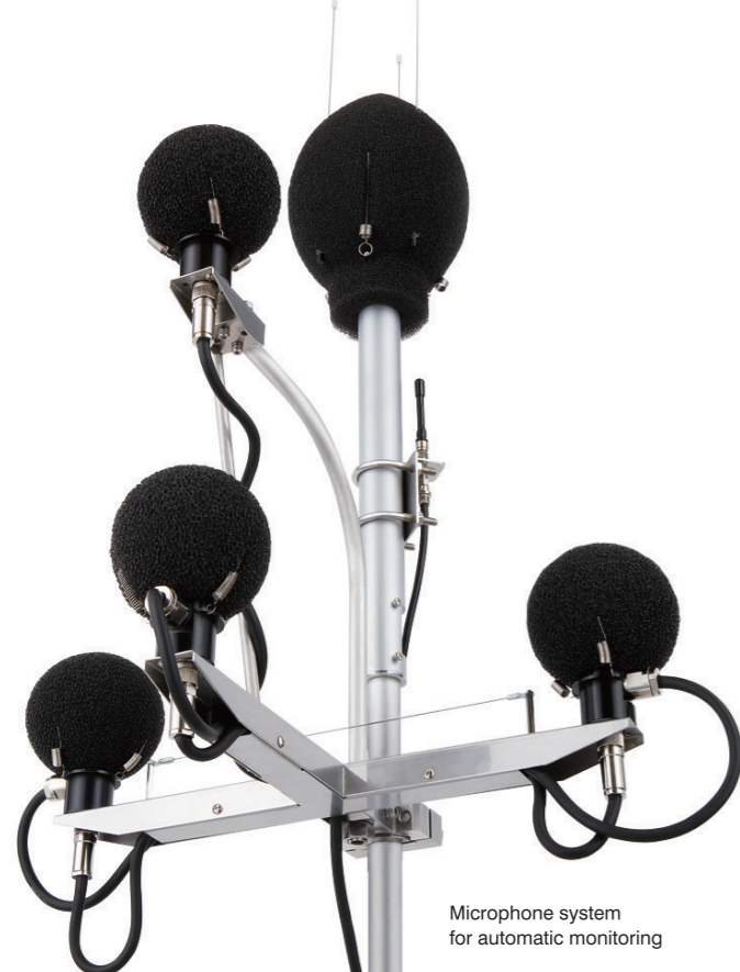
Figure 1: Microphone setting for detecting arriving sound direction
