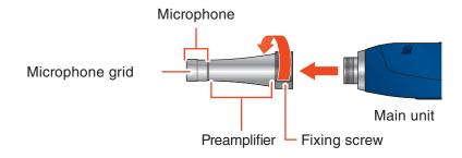
2 Remove the microphone and preamplifier from the main unit.
