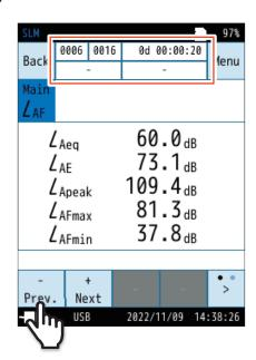
If there are six or more calculated values, on the menu ring, touch [>] and then touch [Disp] to switch to the next screen after the calculated values screen.
