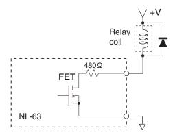
The voltage applied to the relay when the comparator is turned on is per the following formula.
