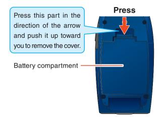
Insert four AA batteries, ensuring that the orientation matches the "+" and "-" marks.
