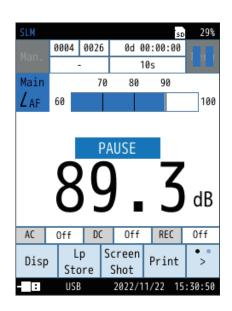
12 Press the START/STOP key to end the measurement.
