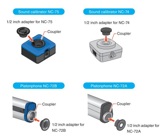
Gently and slowly push the microphone of the device until it hits the back of the coupler.
